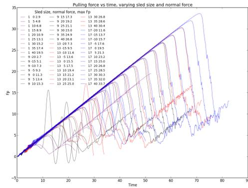
Figure 3: Comparing  $F_p$  vs time for all sled sizes and normal forces shows how similar each simulation run is. Note the erratic oscillations in the early times - these were due to negative normal forces causing the sled to fly away after exceeding  $f_s$ .
