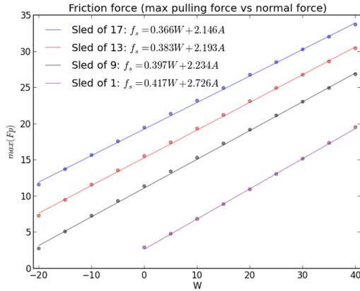
Figure 2: A plot of  $\max(F_p)$  vs normal force for several sled sizes, as well as linear least-squares fits, show that the coefficient of friction and area multiplier vary a bit.
