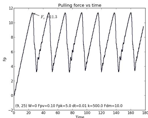
Figure 1: A lengthy run of the simulation shows that the pattern of increasing the pulling force until a breaking point is reached is periodic.
